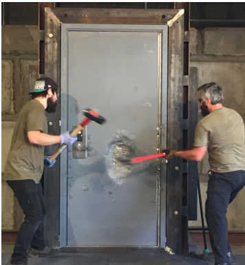
Image from actual forced entry testing
